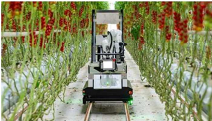
Automated harvesting robot for mini-tomatoes
